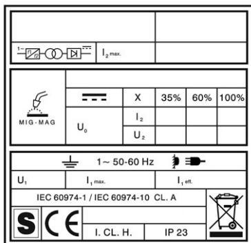
IEC60974-1 The welding machine is manufactured according to these international standards.
